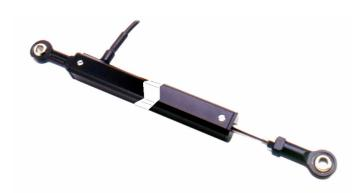
The output of a linear potentiometer is a voltage which changes in direct proportion to the shaft extension. A constant voltage is required across the supply and ground wires of the sensor. Various lengths of electrically active track are available, up to a maximum of 252mm. The sensing elements are made from conductive plastic with a precious metal wiper. The units are sealed to keep out dirt and dust.
